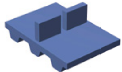
Figure 6.5.4: Rectangular cleats, arranged in series
